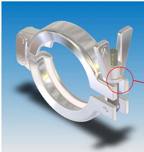
The 'gate' style section combined with the stepped eyebolt assures the clamp's bolting mechanism cannot swing open while the clamping union is part or fully assembled.
