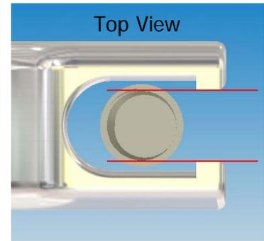
Releasing the clamp is only possible when the wing-nut has been significantly loosened to enable the smaller diameter of the eyebolt to swing and pass through the sectioned gate, this ensures the clamp cannot be knocked or accidentally opened. Complete wing-nut removal is not necessary to open the clamp since the design guarantees the eyebolt cannot swing open while the clamping union is subjected to either clamping forces or internal pressures.
